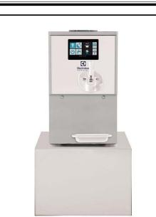
560062 (CAP114DGA3PH) Soft ice cream dispenser with 12 I tank capacity and 1,95 I cylinder volume, 1 flavour, electronical control and touch screen panel, countertop, hourly production: 240 cones (75 gr), gravity version, R452A
